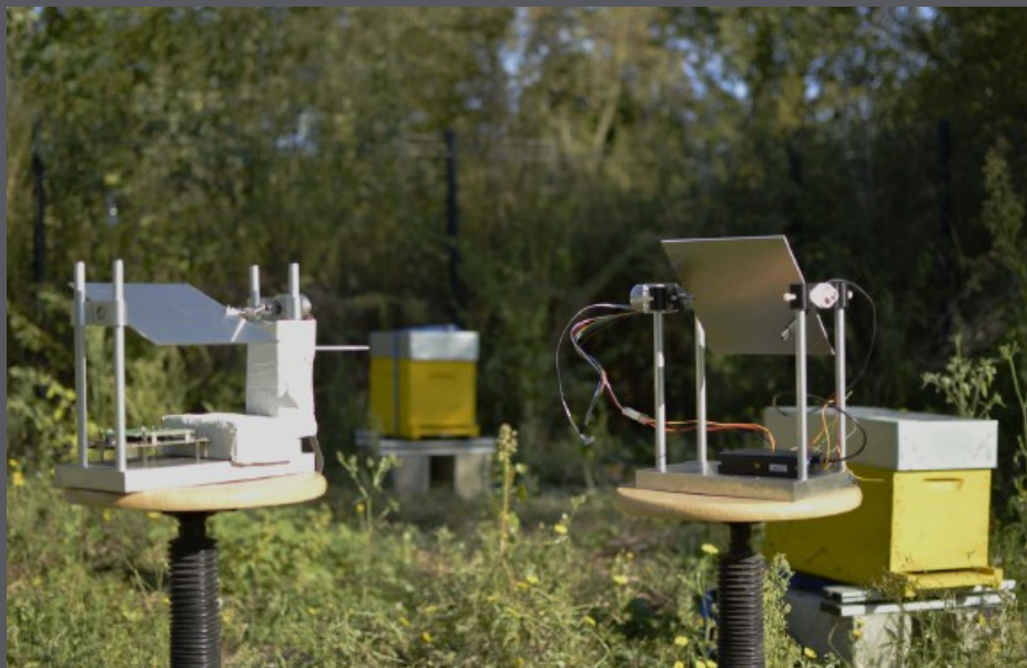
Figure 1: Radar-based tracking system to study bee movements. Left: complete system with radar, support and rotating reflector. Right: system without radar. Photo credit: Tamara Gomez-Moracho.
